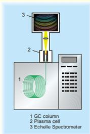
Fig. 2: Scheme of the EPED-detector coupled with GC
